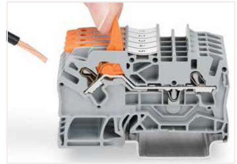
Pull the lever up until it stops, then connect the stranded conductor.
